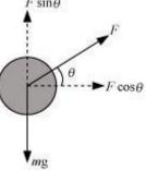
While pushing a lawn mower, a force at an angle  $\theta$  is applied on it. The vertical component of the applied force acts in the direction of the weight of the mower. This increases the effective weight of the mower.
