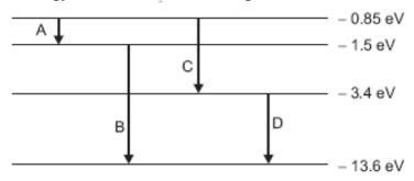
Identify, using necessary calculations, the transition, which corresponds to the emission of a spectral line of wavelength 482 nm.  $[B(\Delta E=2.55eV)]$
